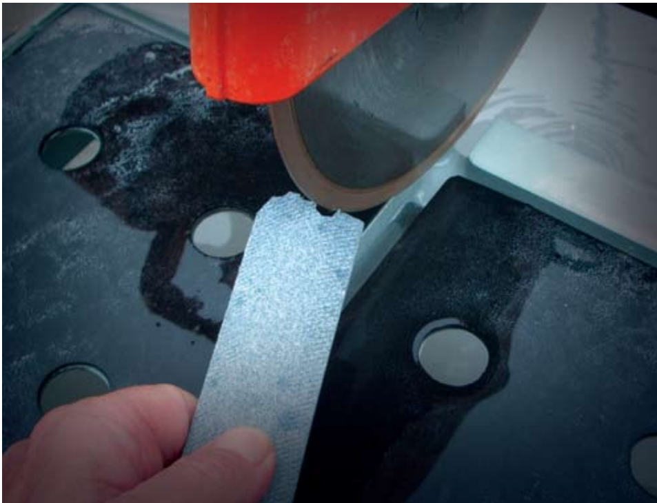
Using a carborundum dressing stick to clean and refresh the saw blade.
